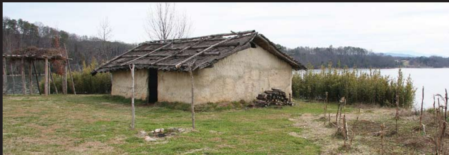
Reproduction of a late 1700s Cherokee house made of wood and clay daubing. Note the rivercane behind the house on the river bank. Rivercane, one of the most important natural resources to the Cherokee, was once abundant along most western North Carolina streams.
